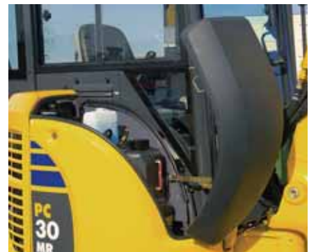
Front bonnet: fuel tank refilling
