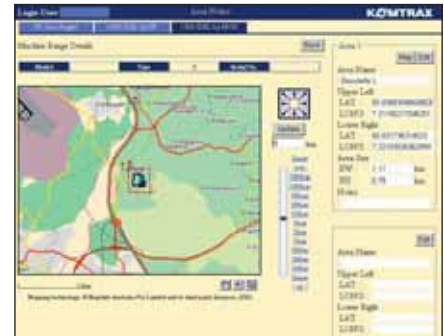
Added security - The "engine lock" feature allows to program when a machine's engine can be started. And with "geo-fence", KOMTRAX™ sends notification every time your machine moves in or out of a predetermined operating area.
